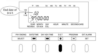
(1) Press  $\frown$  or  $\frown$  to cause digits to flash, and then press  $\frown$  or  $\frown$  to select the desired time.
