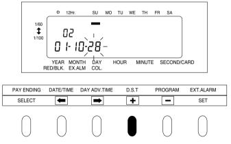
(2) Check the settings on the display and press SET. Now the setting is completed.
