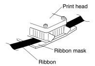
NOTICE: Install the cassette so that the ribbon is between the print head and the ribbon mask. Printing will not come out properly if the ribbon is placed behind the ribbon mask.
