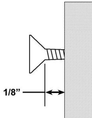
2. Install screws (included) at positions B and C with 1/8" gap between the screw head and wall. Install screw anchors (included) if necessary.
