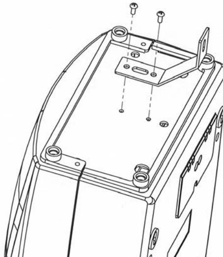
4. Line up the keyholes on the back of the T100 with the mounting screws. Slide the T100 downward to secure it to the wall.
